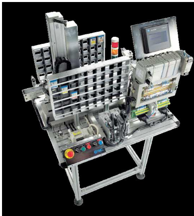
Figura 7. HAS-208 - Almacén vertical
