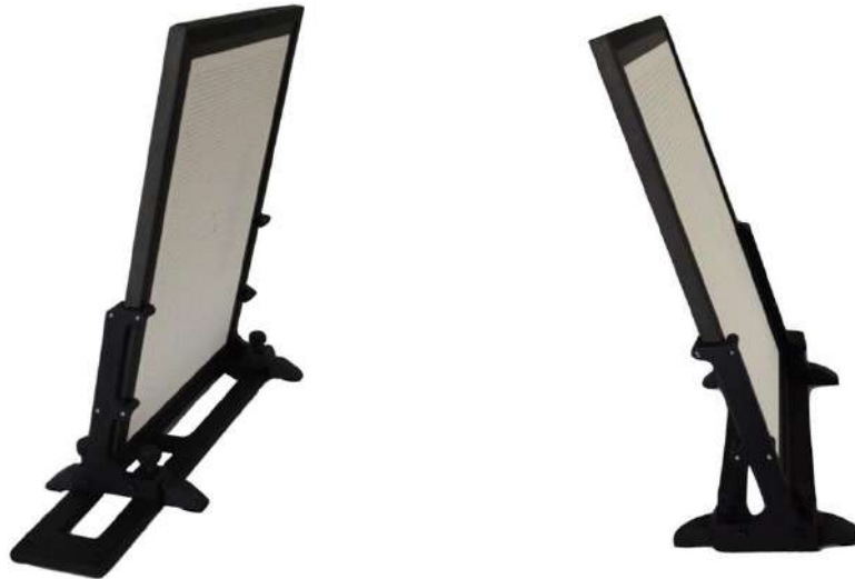
Fig. 6-36. Correct installation of the tilted calibration table forwards and backwards for the outer range
