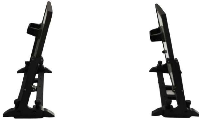
Fig. 6-19. Correct installation of the tilted calibration table forwards and backwards for the inner range
