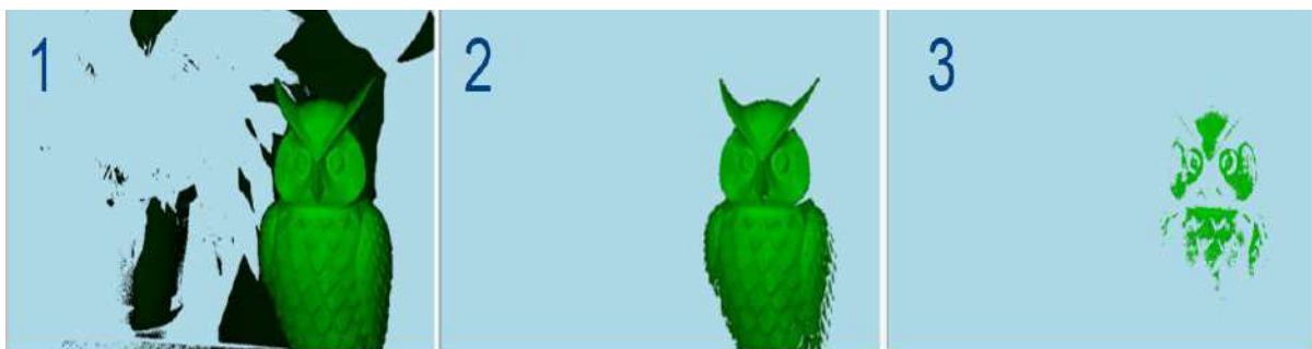
Fig. 5-30. Example of the view for different shade level settings: 1 – value 10, 2 – value 80, 3 – value 160.
